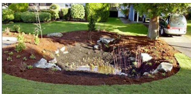
Example of residential rain garden. Darker mulch is contained within the allowable ponding zone of the rain garden.
